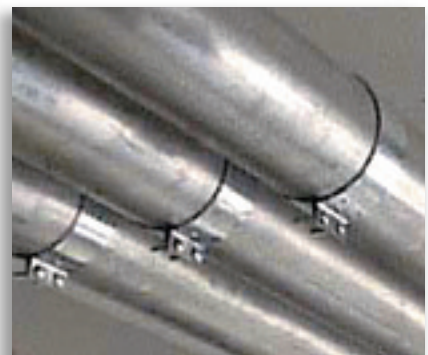
Colombo BeverageChase® System is smooth inside for easy pull through. Joint strength holds the weight of multiple lines and withstands pull-through stresses.
